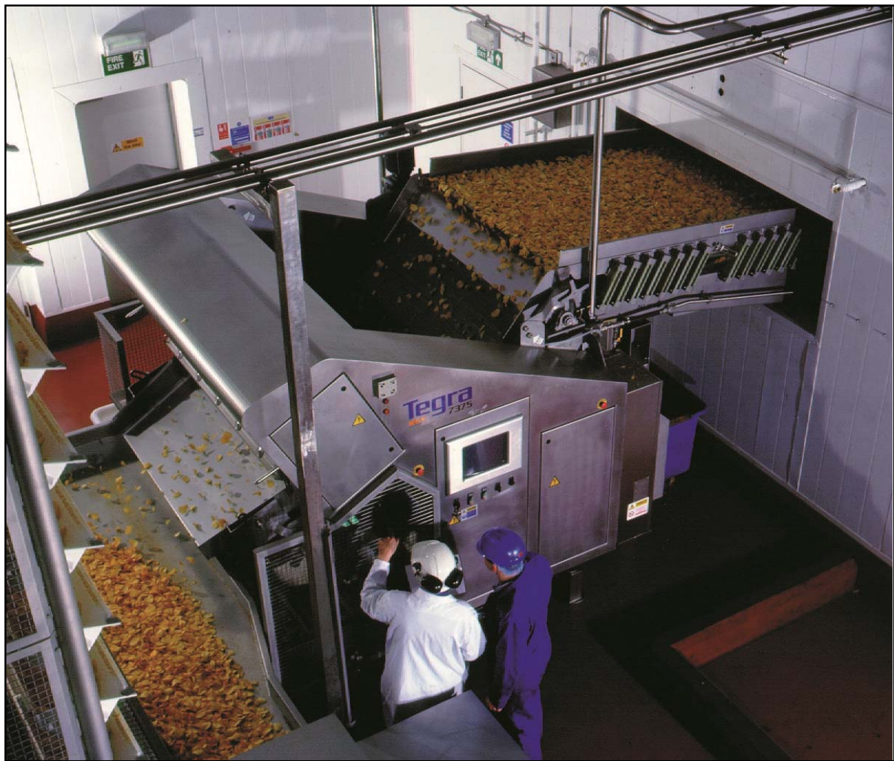
An optical sorter removes burnt, broken and otherwise objectionable potato chips
