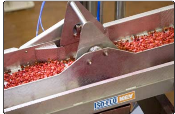
This Iso-Flo vibratory shaker incorporates a swing gate for distribution of in-process Craisins.
